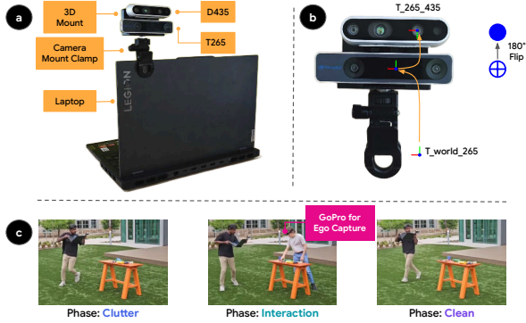
Fig. 3: Capture setup. (a) D435 + T265 rig on a laptop mount, carried by hand. (b) Sensor detail with the T265→D435 extrinsic and world→T265 pose frames. (c) Three phases of one scene; the GoPro is visible during Interaction; faces blurred for anonymity.
