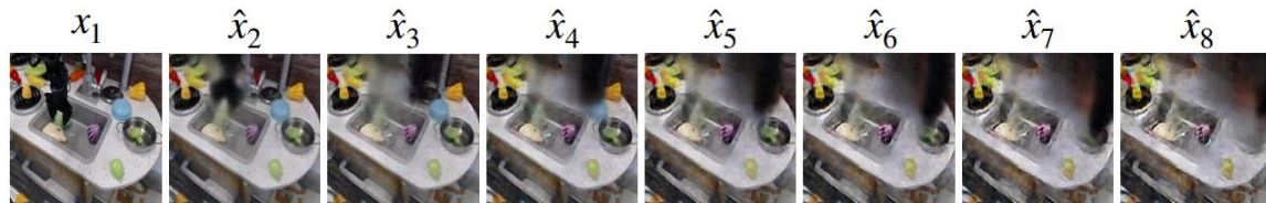
Figure 12: Closed loop rollout of LAPA. LAPA is conditioned on current image x_1 and language instruction of 'take the broccoli out of the pot' . We generate rollout images by conditioning the decoder of Latent Action Quantization Model with latent actions generated by LAPA.
